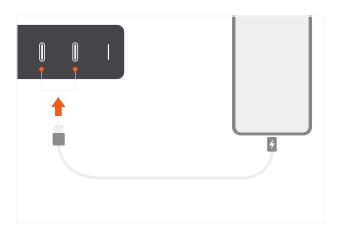
2 Power a USB-C laptop by connecting to one of the charger's PD ports - up to 100W with a single device connected.
